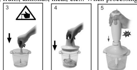
Place the lid by hooking it to the appropriate joints on the container, as shown in **Figure 4**.
